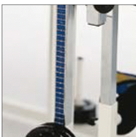
Height adjustable load arm with reference scale.
